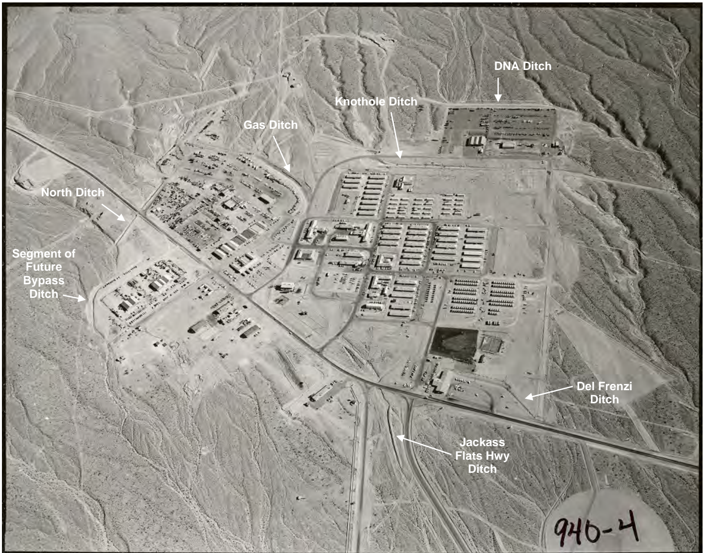
An aerial view of Mercury before the implementation of the master plan (ABA 1962) showing some of the more prominent natural and constructed drainages, facing east (REECO, January 1961).
