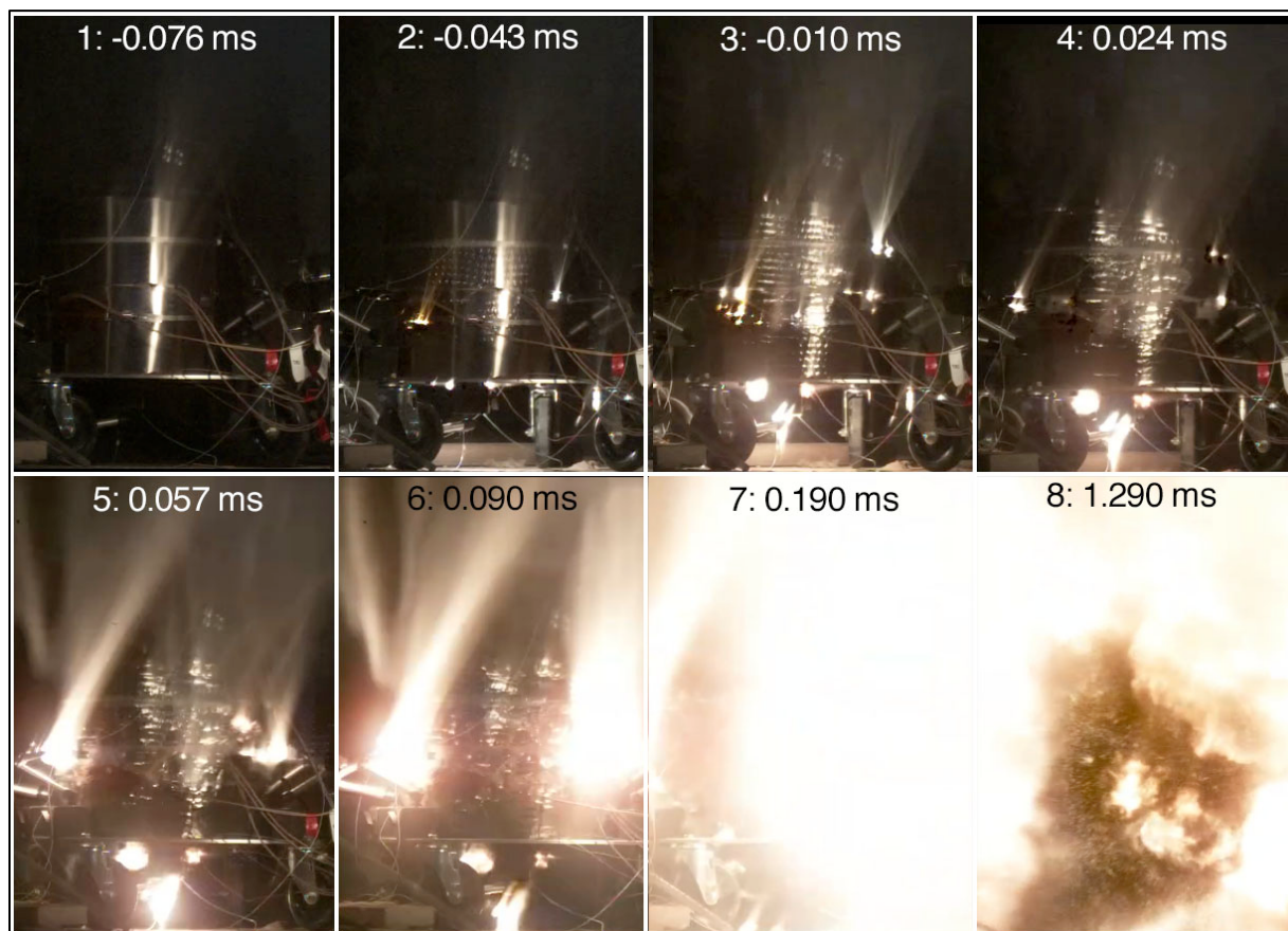
Figure 37. SITX (Test 3) still sequence from high-speed video record. Video was captured as 20,000 fps. Insulation and metal flashing is wrapped around the shot and obstructs the view of the fracturing metal surface that is visible in the first two experiments. The view is blurry because rain collected on the glass porthole in the middle of the night; the camera was looking through a puddle of water.
