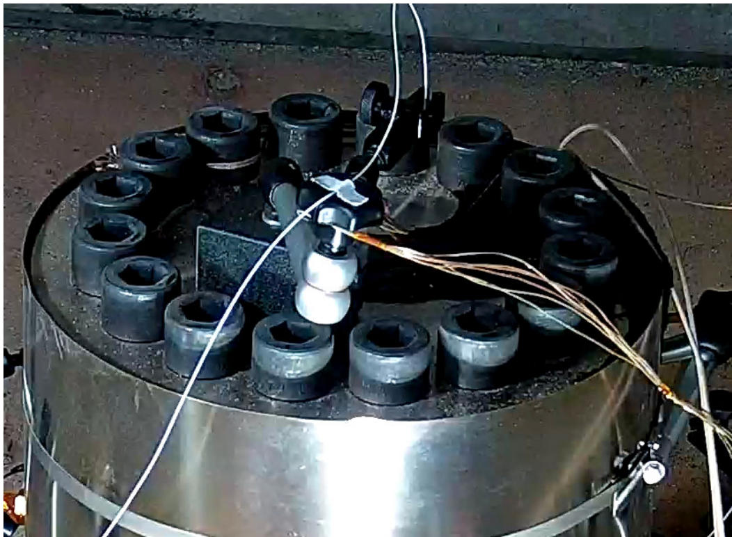
Figure 24. Binder expelled from top feedthrough is visible on lid in this still frame from surveillance video during the test.
