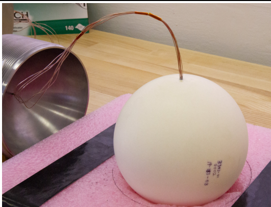
Figure 28. Interior thermocouples potted into charge.
