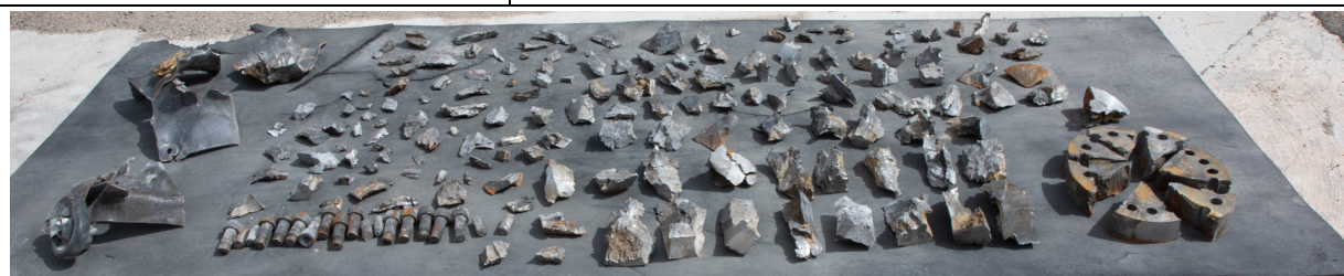
Figure 16. Photograph of all the fragments that were collected from LIPX.
