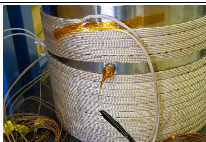
Figure 31. Feedthrough mounted in vessel; heating tapes partially wrapped.
