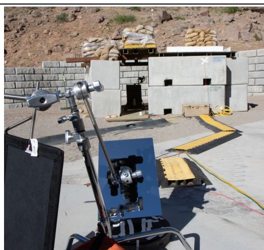
Figure 10. View from behind porthole, showing the angle from which the high-speed video is viewing the shot. Both turning mirrors are visible in the photograph. Mirror in the foreground is directly over the porthole. Dark square visible in block house opening is the second turning mirror.
