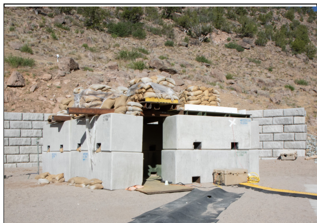
Figure 9. Block house before explosion. Blocks and sandbags are mitigation to prevent hot fragments from escaping mound to potentially start fires in surrounding landscape.
