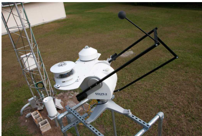
Sun tracker measures irradiance at the FL RTC
