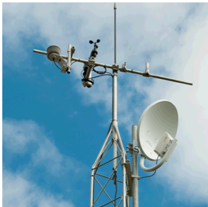
Weather instruments on top of 30m weather tower
