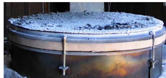
Post-test Calorimeter with Deposit
