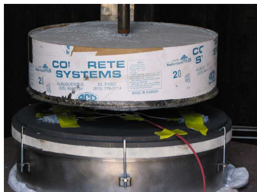
Downward-facing Propellant Charge Held Above Calorimeter
