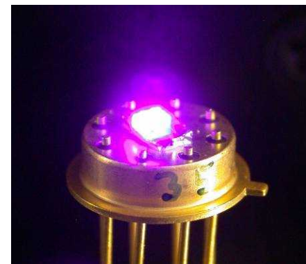
Sandia flip-chipped InGaN LED on TO-header
