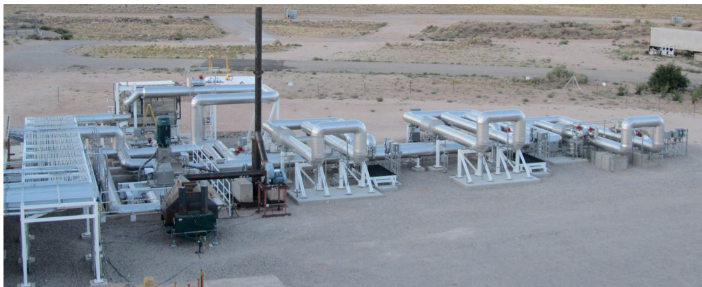
The Molten Salt Test Loop has three parallel test sections for simultaneous customer solar component testing. MSTL is the only test facility in the country that can provide real power-plant conditions and collect data about the interactions of pressure, temperature, and flow rates. (Photo by Randy Montoya)
