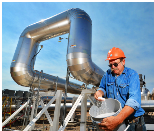
Sandia mechanical technologist John Kelton sifts through a bucket of salt beads before they are melted for use in MSTL. When a customer wants to test using MSTL, the vertical loop shown here is removed and the customer's experiment is put in place of the loop. Customer experiments can be as small as testing instrumentation on materials, or as large as on-sun testing of concentrating solar collection modules. (Photo by Randy
