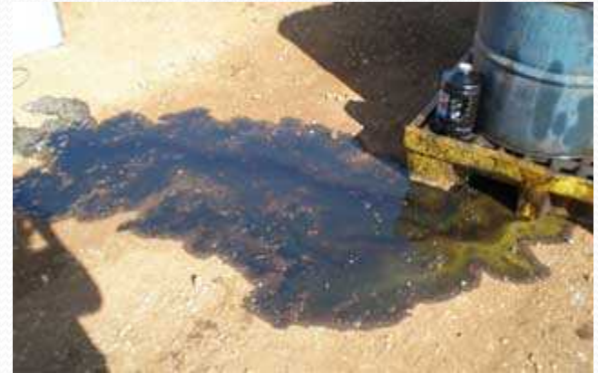
Leaky drums without secondary containment.
