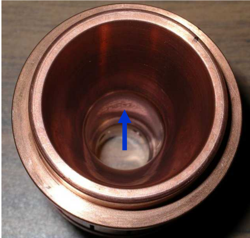
1 st run 0.5" arc chamber, 0.41" throat: 23 minutes
