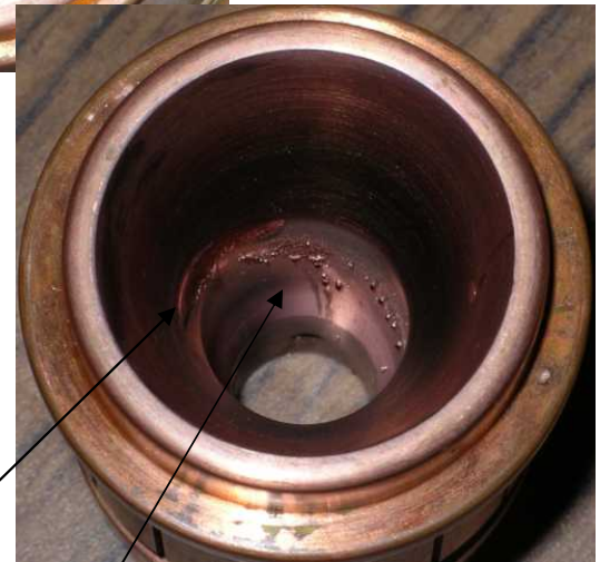
Arc chamber still intact and showing little wear
