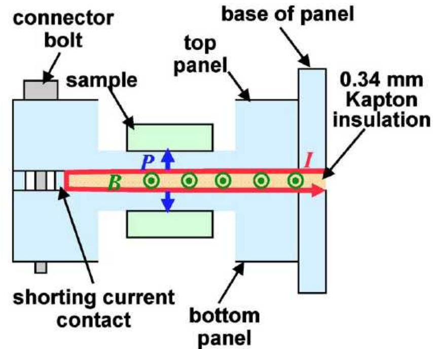
Strip-line design allows for samples to be placed on both the anode and cathode, and thus they both experience the same B field
