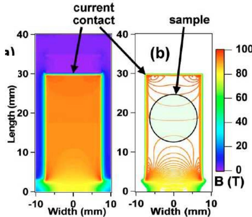
Simple panel design has a field gradient along the panel length
