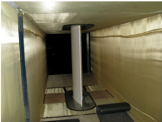
Figure 5: DU97-W-300 model in wind tunnel test section. View is upstream.
