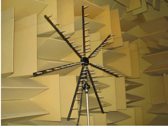
Figure 6: Microphone phased array.
