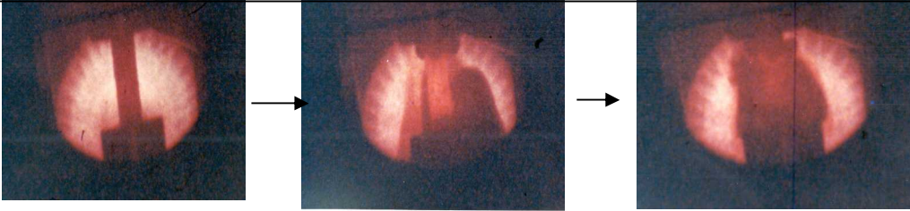
Pin heatup, clad melt and FP release, and fuel disruption sequence in LMFBF high burnup fuel pin (FD Program - JNC, UKAEA, KFK, NRC)
