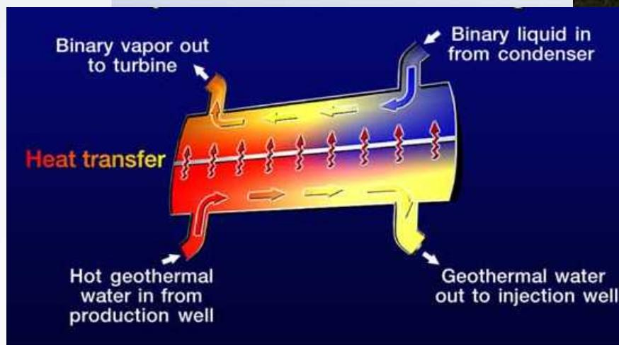
This plate-type heat exchanger passes geothermal water over metal plates for heat transfer to the working fluid on the other side.
