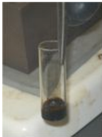
Initial KCl-LiCl- \text{CuCl}_2 molten salt at 400°C
