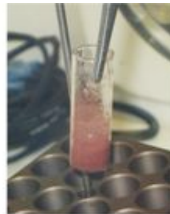
Reddish color resulting from Cu-metallization in KCl-LiCl- \text{CuCl}_2 molten salt at 400°C
