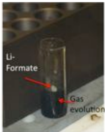
Addition of Li-Formate ( \text{LiCOOH} ) to KCl-LiCl- \text{CuCl}_2 molten salt at 400°C rapidly evolves \text{CO}_2 and \text{H}_2 gases.
