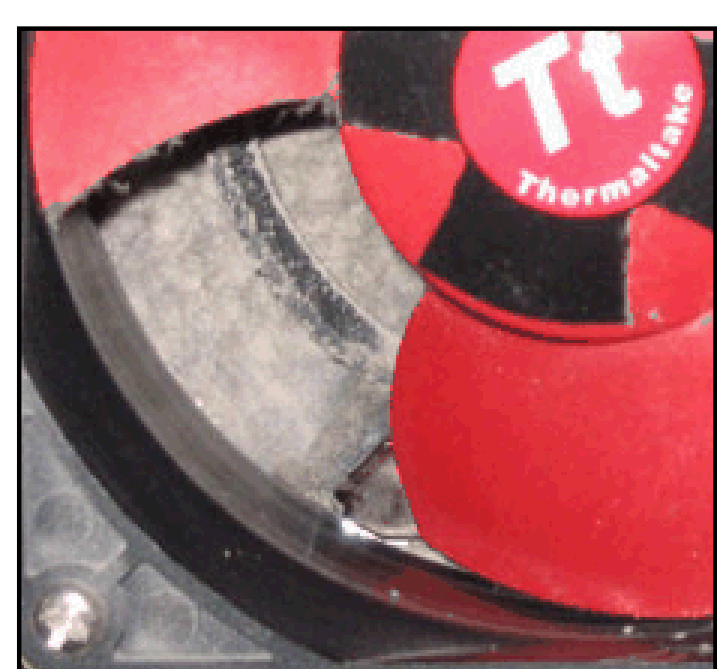
The end result of heat exchanger fouling. Cooling fins are buried in a thick layer of dust, choking off air flow.
