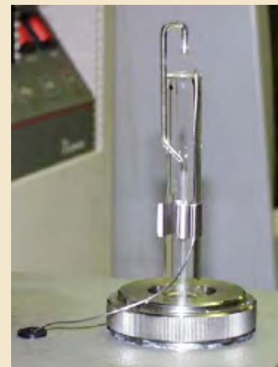
Thermal Mechanical Analysis (TMA) expansion fixture
