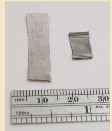
PVDF film before and after shrinkage.
