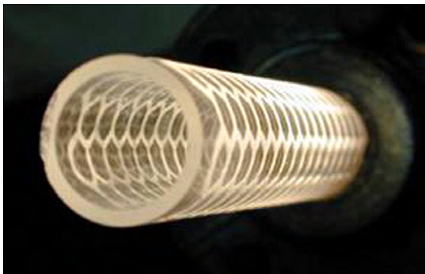
Figure 2: 3D complex shape direct-printed onto a curved substrate. Conductors in this shape become highly sensitive antennas.
