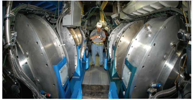
In a tunnel 962 feet below the surface of the Nevada Test Site, Gene Ormond prepares the cathode cover of the Sandia-designed, high-intensity flash X-ray system for weapons certification.
