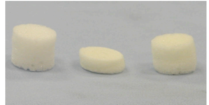
Shape-memory effect in polyurethane foam
