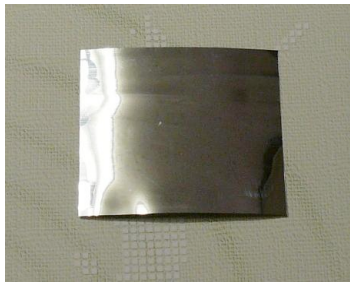
PVDF film metallized on both sides
