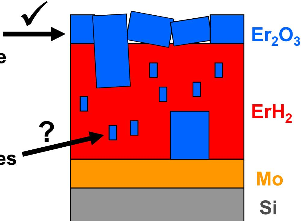
Satellite diffraction spots could be due to nano-oxides within the  $\text{ErD}_2$  matrix
