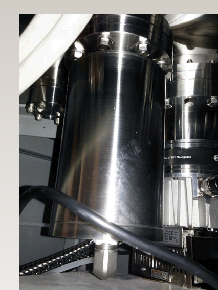
Custom pneumatic actuator
