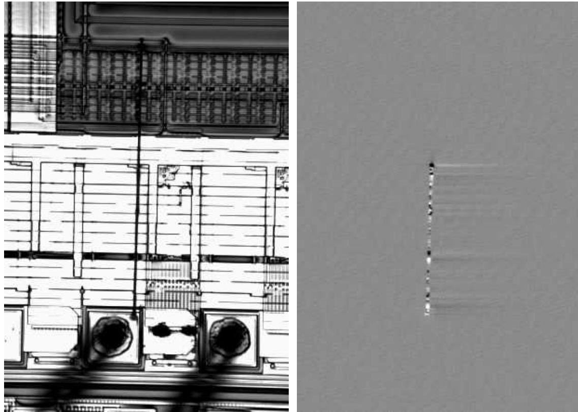
The FIB conductor is shorted to an underlying power bus where the TIVA contrast abruptly stops. No direct bias was applied. The TIVA voltage signals, yielding the black and white speckled pattern, are believed to result from laser heating of "thermocouples" produced from random Pt grains along the deposited line.
