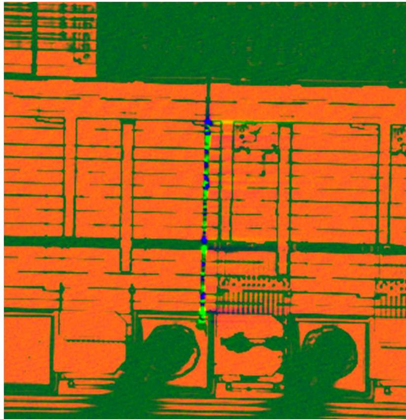
The FIB conductor is shorted to an underlying power bus where the TIVA contrast abruptly stops. No direct bias was applied. The TIVA voltage signals, yielding the blue and green speckled pattern, are believed to result from laser heating of “thermocouples” produced from random Pt grains along the deposited line.
