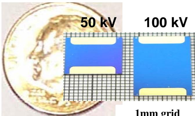
PCSS switch (40 kV, 100A, sub-ns risetime) used to trigger a one stage, 200kV, 20 kA Marx generator under development for DOE/NNSA program
