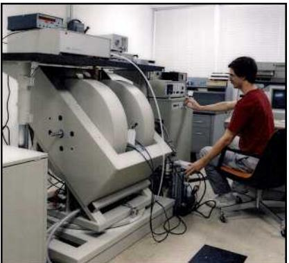
Electron paramagnetic resonance for defect studies
