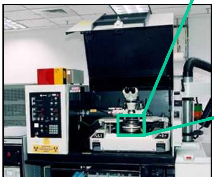
256-channel capacity with integrated IC tester
