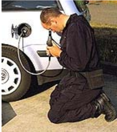
Fiber-optic tool to look inside enclosed spaces
