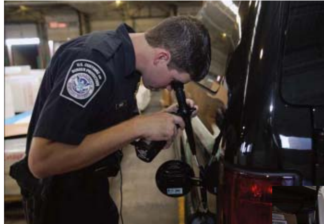
Fiber-optic tool to look inside enclosed spaces
