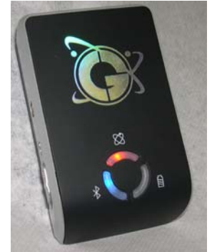
Bluetooth GPS Receiver for added geo-tagging capability
