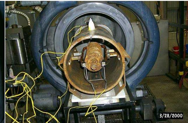
FSS and conical shaped charge
