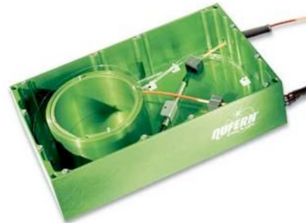
The mode filtered fiber amplifier, developed jointly by Sandia and the Naval Research Laboratory, is used extensively in commercial fiber lasers.
