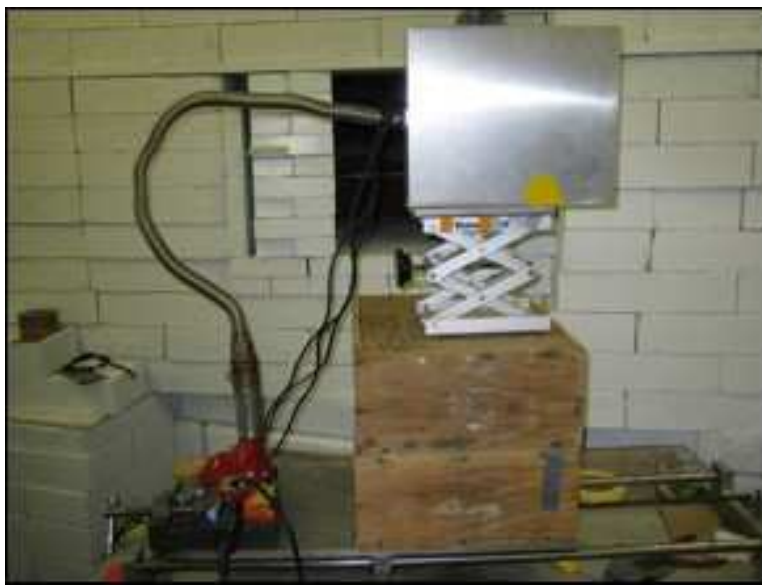
Fig. 3. Portable environmental chamber for testing devices at elevated temperature. The DUT is located inside the heated chamber.
