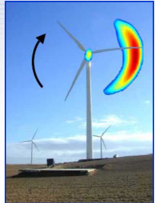
Noise map on a 850 KW turbine from the European SIROCCO project.
