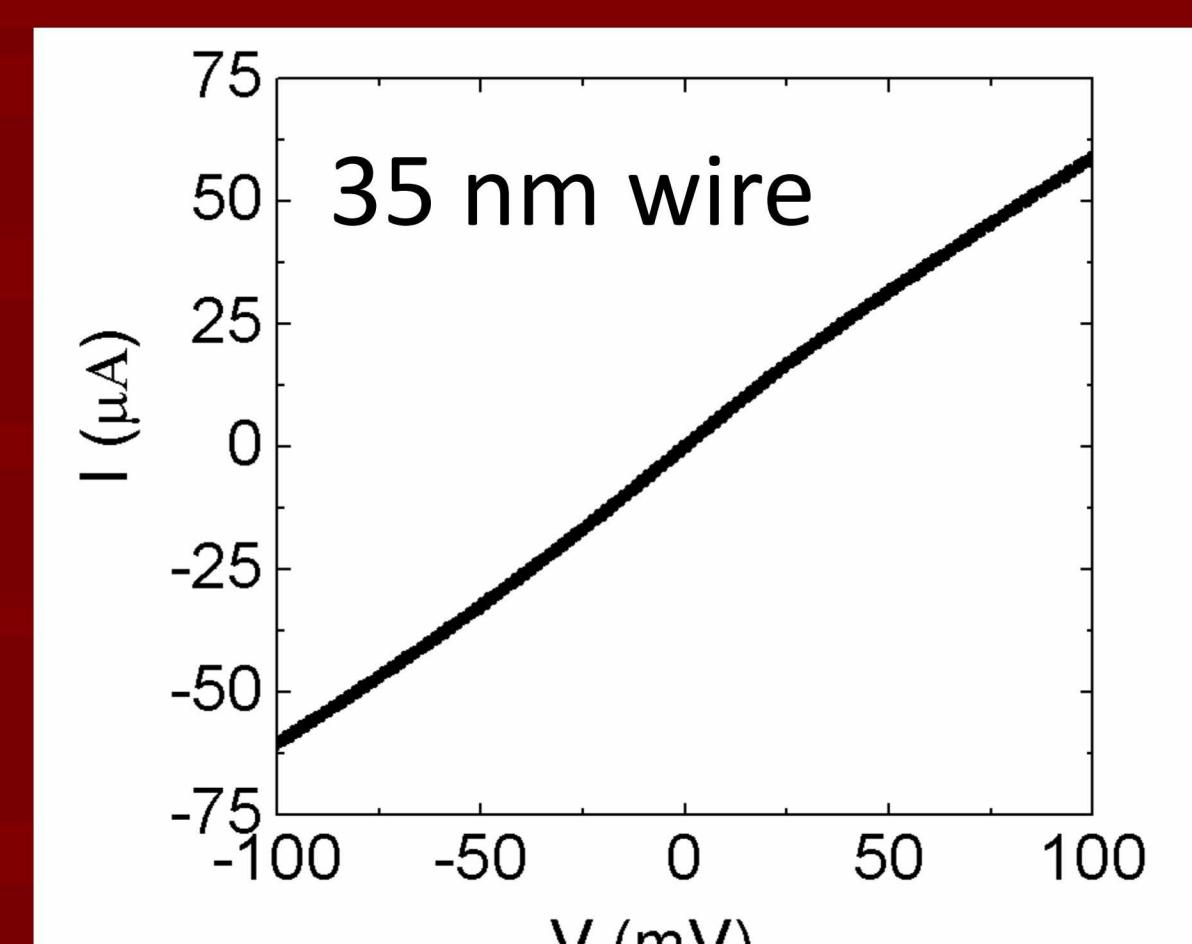
AP nanowires can achieve high current density  $\sim 2 \text{ mA}/\mu\text{m}$  at cryogenic temperatures
