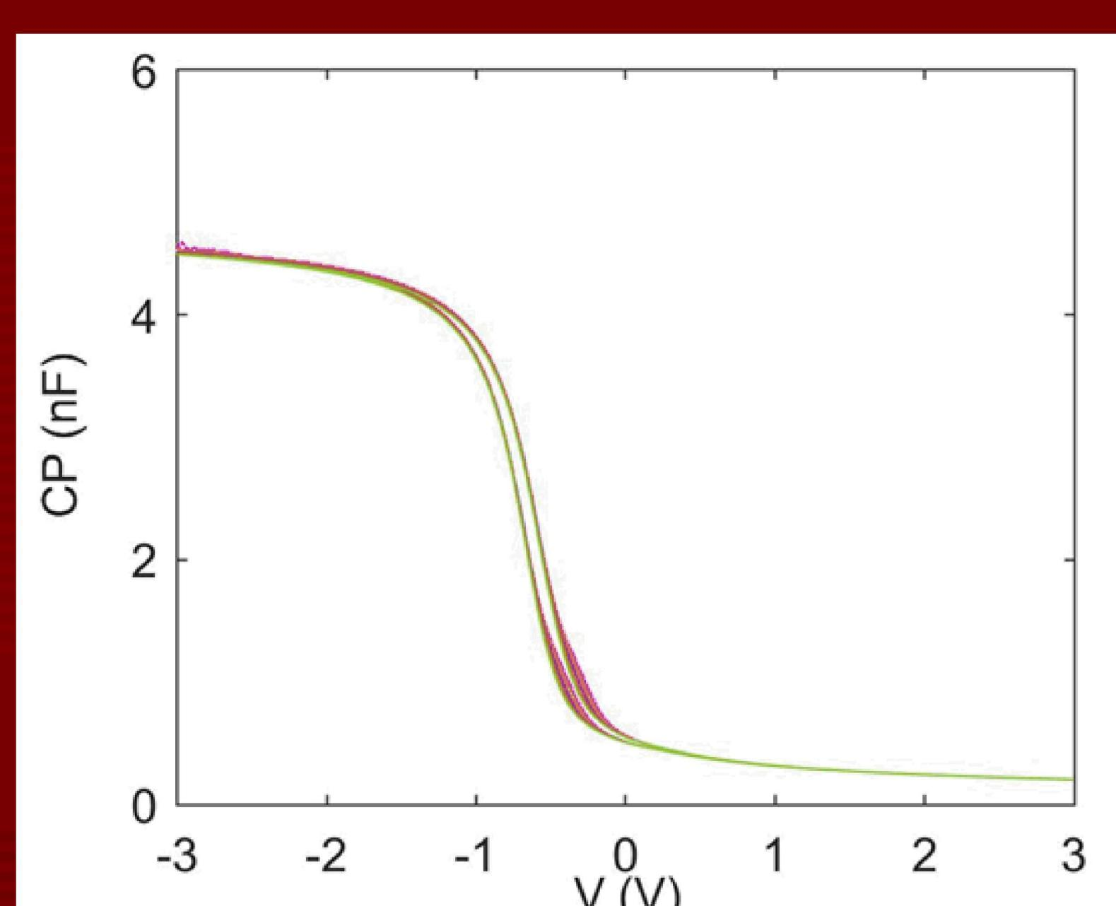
High-k dielectric: We have a low thermal budget gate stack with  $\sim 10^{11}/\text{cm}^2$  defect density at RT
