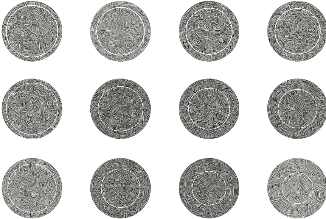
Fig. 5. Streamlines in cross-sectional planes (evolution of quasi-streamwise vortex patterns). Top = Run 618U, middle = Run 635U and bottom = Run 445U. Left to right: x = 0D, 5D, 15D and 25D . White solid circles denote the locii where the mean value of y_w^+ is thirty.
