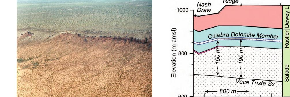
The Culebra is vertically heterogeneous, exhibiting different amounts of vugs and fractures, locally filled with sulfate and/or halite cements. It has multiple types of porosity at different scales.
