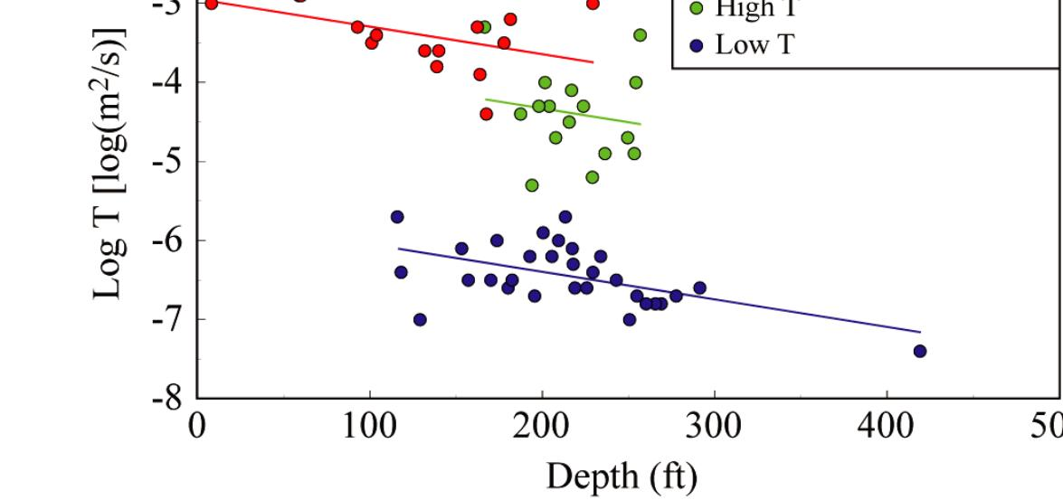
A fourth factor, halite bounding (and cementing) the Culebra, causes much lower T east of the Rustler mudstone-halite margins.
