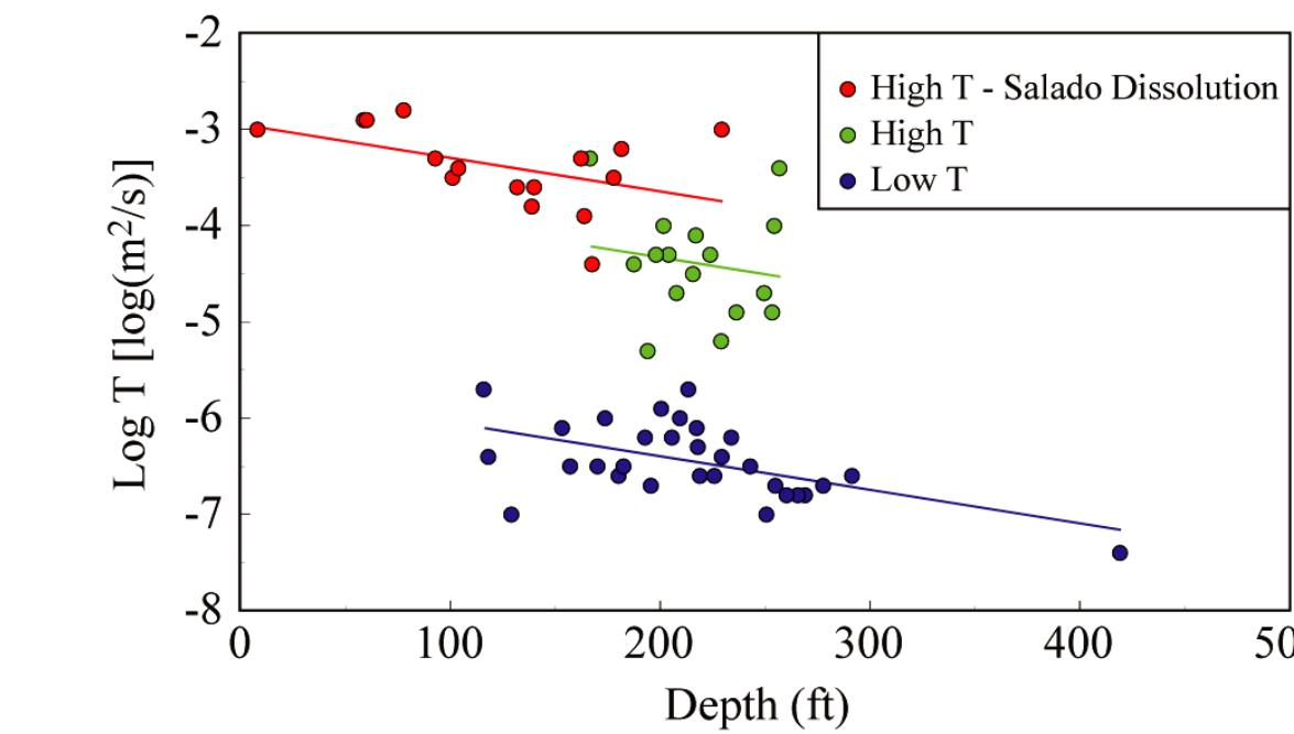
A fourth factor, halite bounding (and cementing) the Culebra, causes much lower T east of the Rustler mudstone-halite margins.
