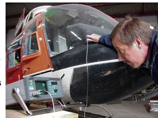
Corrosion Detection with Dual Frequency Eddy Current
