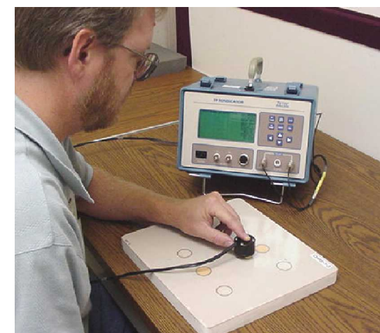
Corrosion Detection with Dual Frequency Eddy Current
