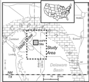
Figure 1. The WIPP is situated in the northern portion of the Delaware Basin, which underlies south-eastern New Mexico and portions of West Texas. The repository is excavated in bedded halite of the Salado Formation, approximately 655 m below ground surface.
