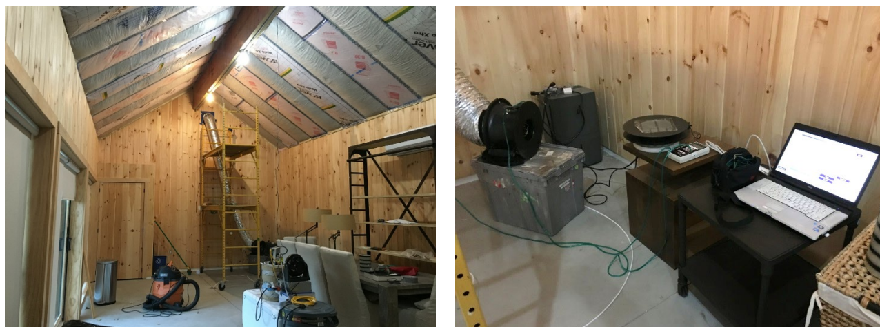
Figure 171. Airtightness testing with fan connected to exhaust fan opening
