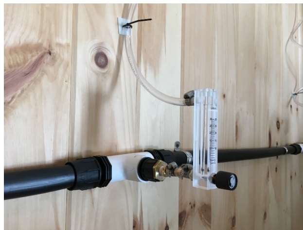
Figure 187. Shop vacuum used as blower (left); rotameter and tubing connection (right)
