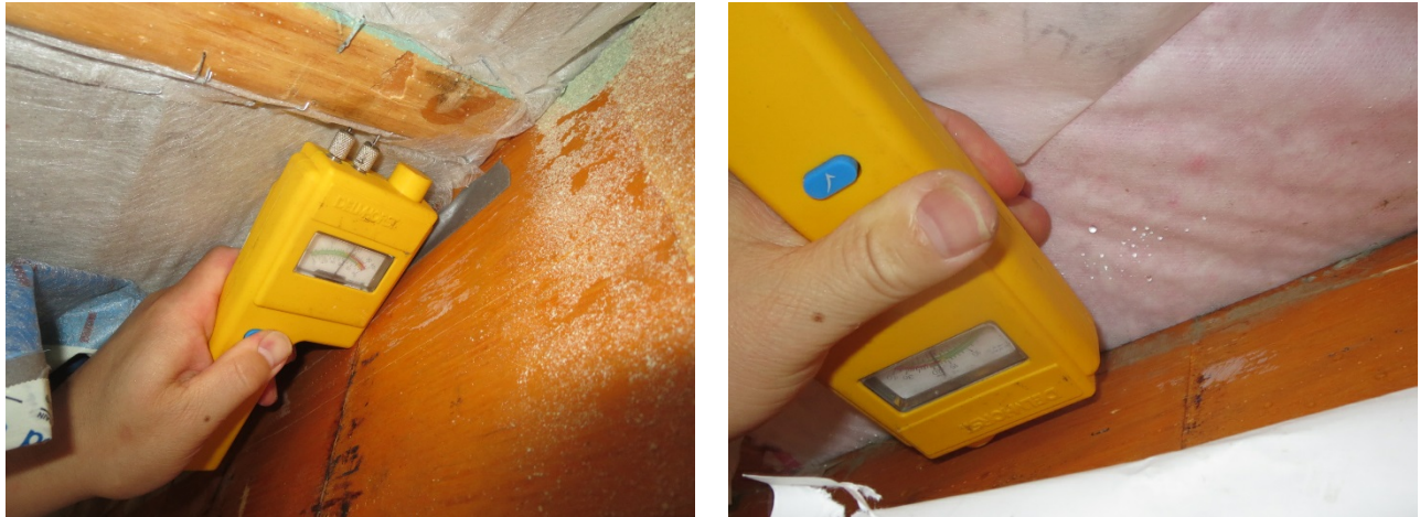
Figure 136. Wood MC measurements at framing
