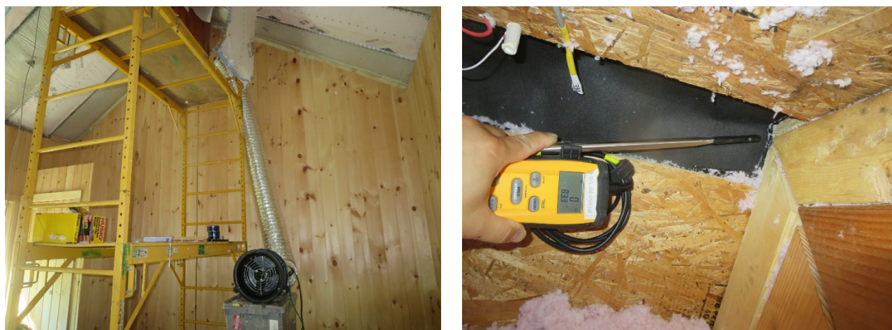
Figure 168. Test hut depressurization (left) and airflow measurement at diffusion vent (right)
