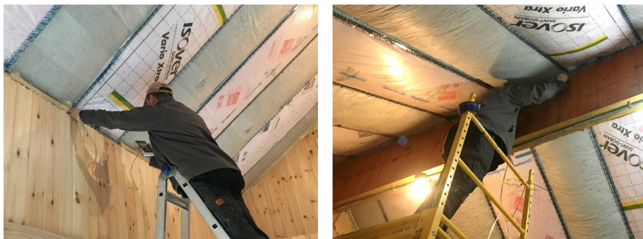
Figure 176. Measuring \Delta P across air/vapor control membrane at eave (left) and ridge (right)
