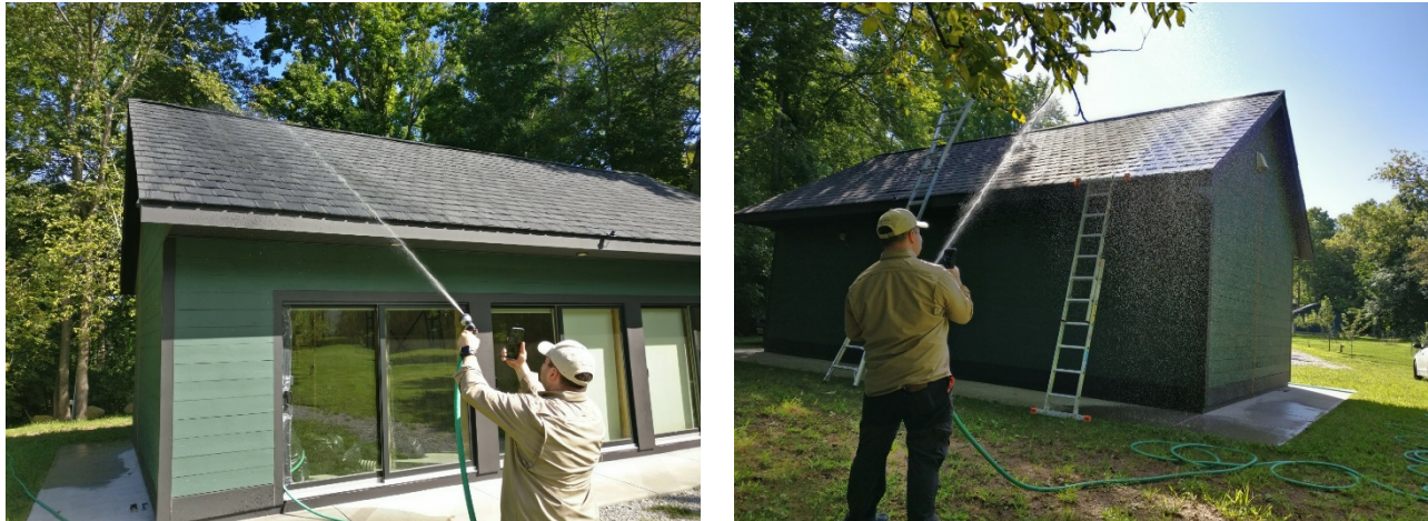
Figure 169. Hose spray testing of roof ridges with interior observation
