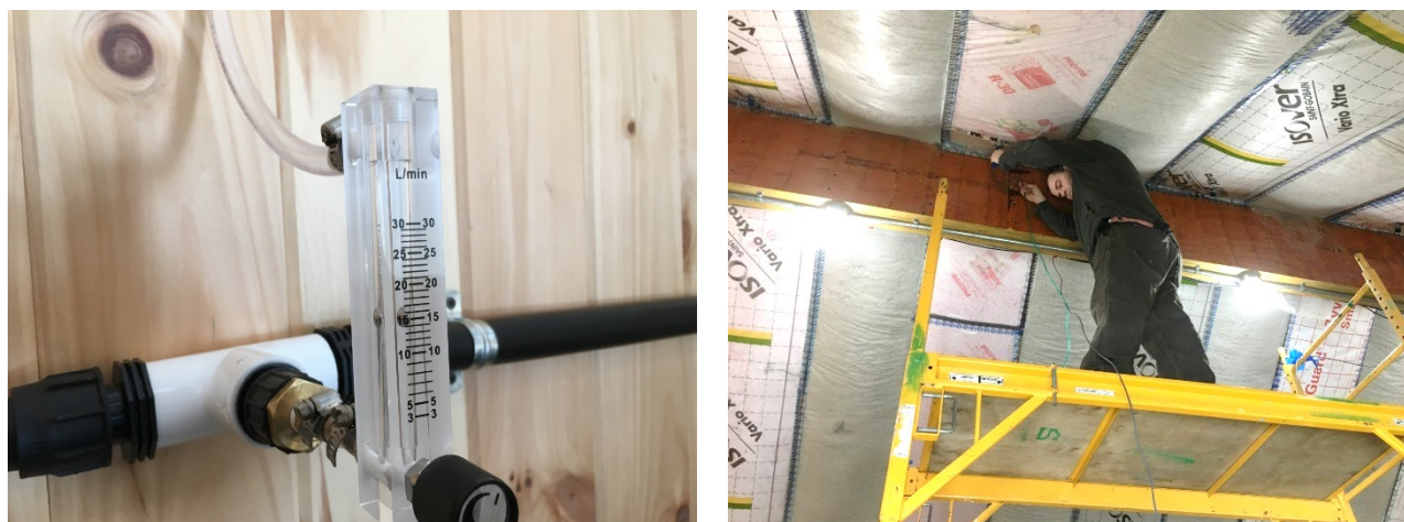
Figure 190. 15 liters/minute airflow rate (left), measuring pressure difference at relief opening (right)
