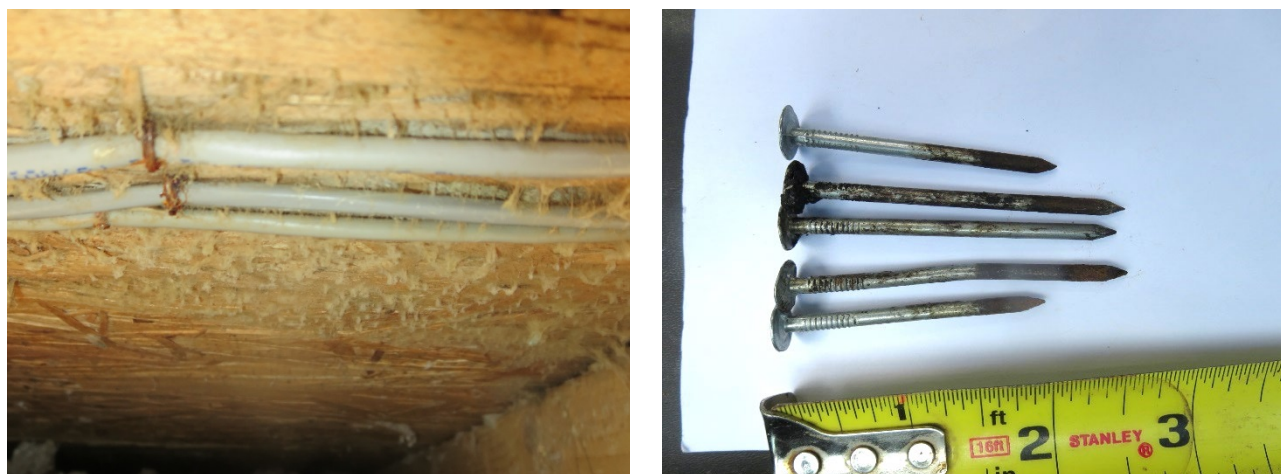
Figure 147. Corrosion of wire staples (left) and corrosion of roofing nails (right)
