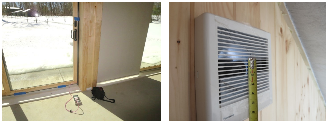
Figure 113. Door opening to relieve pressure (left), exhaust fan restriction (right)
