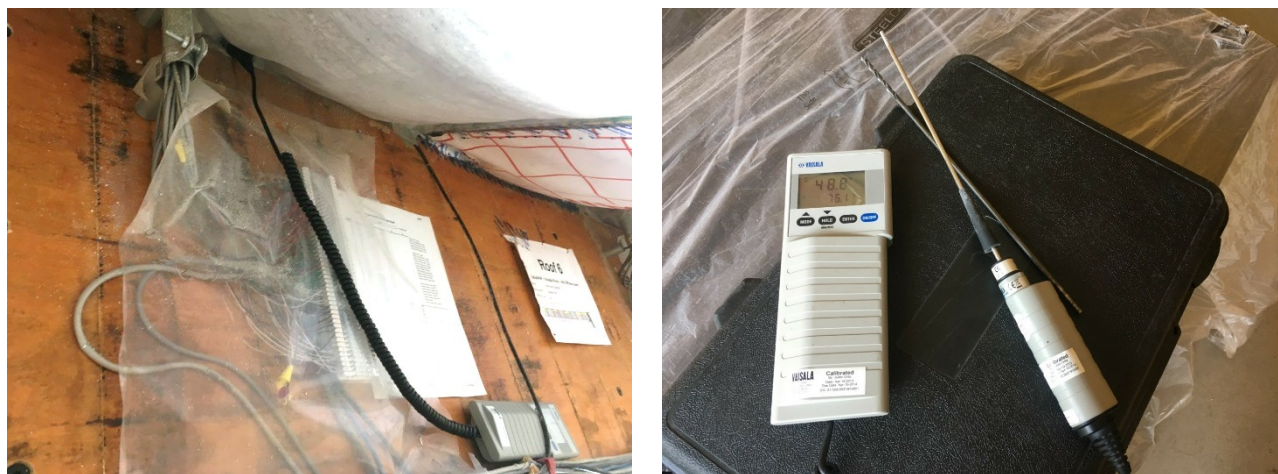
Figure 98. Measurement of T/RH at ridge using Vaisala probe
