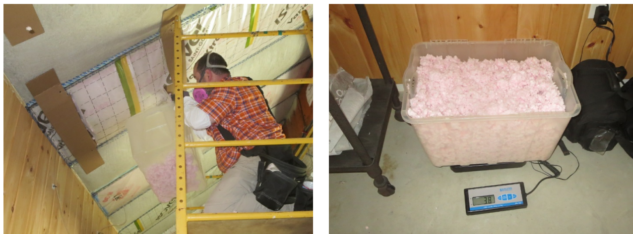
Figure 197. Removal of fiberglass for density measurement and weighing
