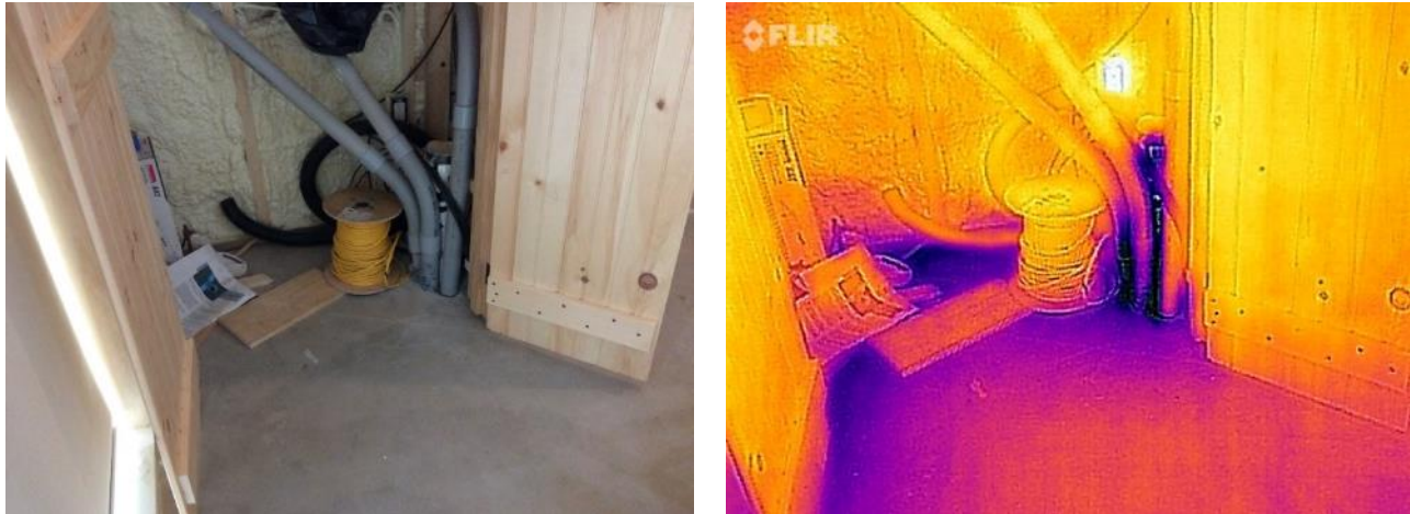
Figure 116. Visual and infrared image of conduit penetration at slab, depressurization test
