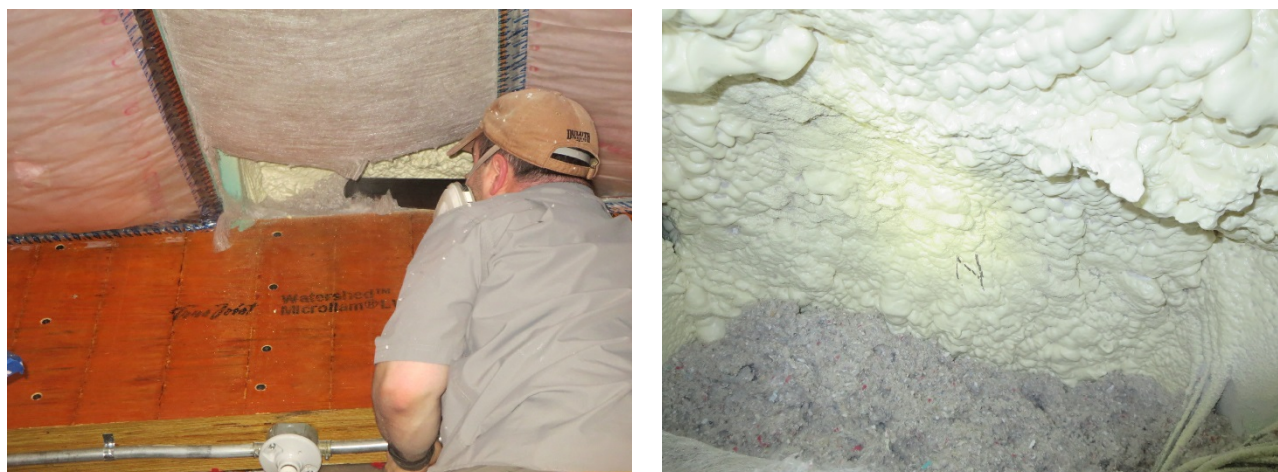
Figure 167. Disassembly of guard bay (hybrid ccSPF-cellulose) ridge and examination
