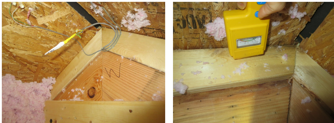
Figure 157. Roof 4 mostly clean conditions on west rafter (left) wood MC measurements (right)
