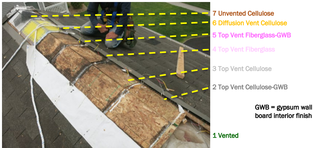
Figure 1. Disassembly of Chicago unvented roof assemblies at conclusion of experiment
