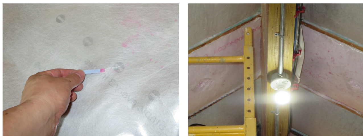
Figure 134. Roof 3 condensation wicking into water indicator paper, staining of insulation netting
