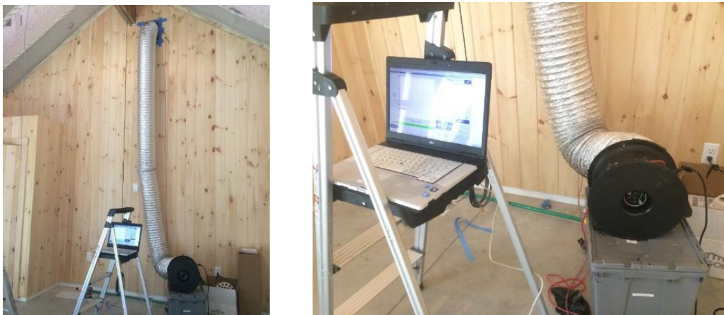
Figure 110. Airtightness testing with fan connected to exhaust fan opening
