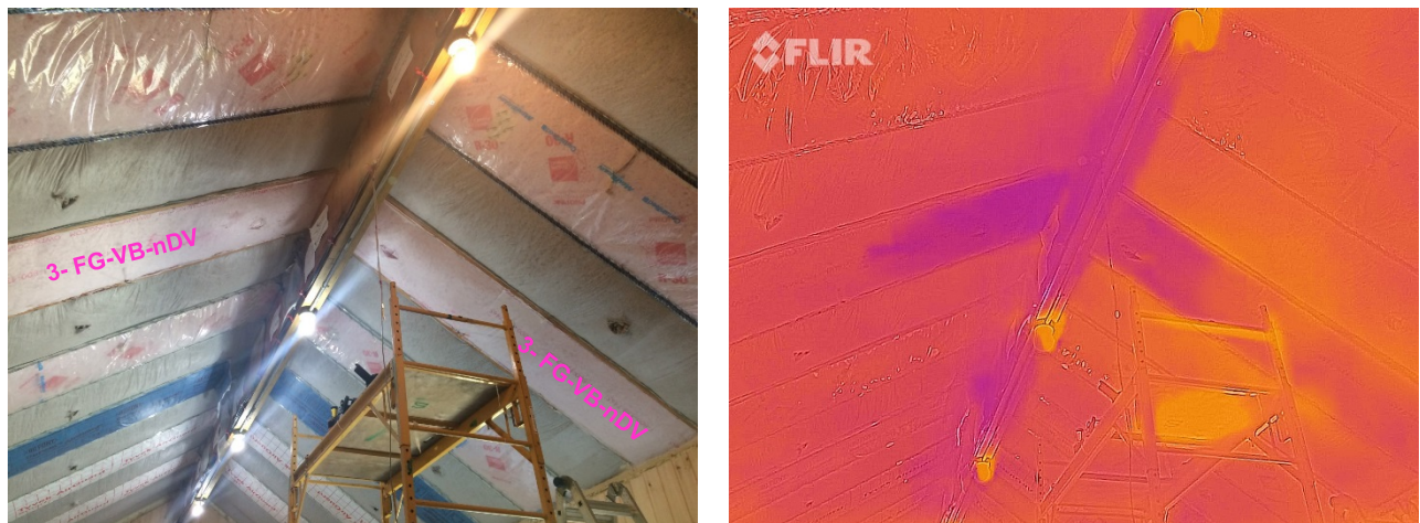
Figure 137. Visual and infrared image of Roof 3 (fiberglass) after fixed-perm vapor retarder removal
