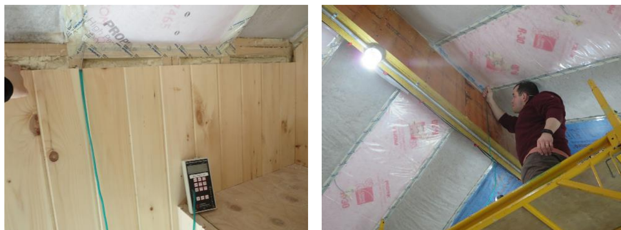
Figure 120. Measuring \Delta P across air/vapor control membrane at eave (left) and ridge (right)
