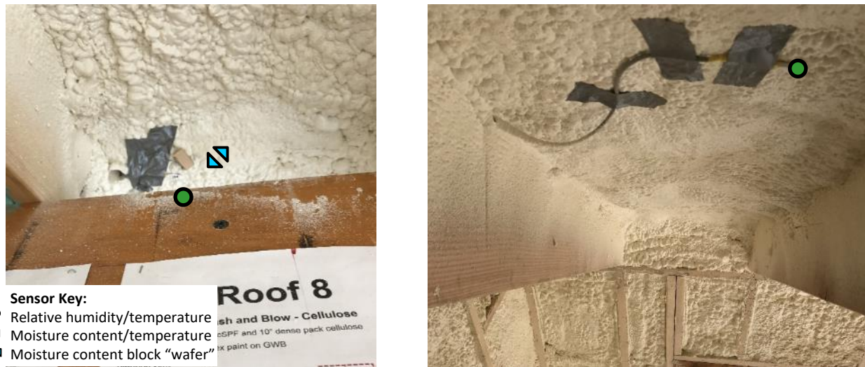
Figure 32. ccSPF-cellulose interface sensors at ridge (left) and mid-height (right)
