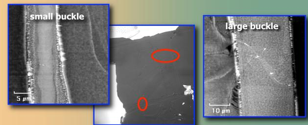
The cohesive zone simulations accurately describe the change in buckle morphology with film stress, providing a lower bound to seemingly disparate sets of data
