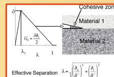
Cohesive zone elements were inserted along the initial portion of the interface
