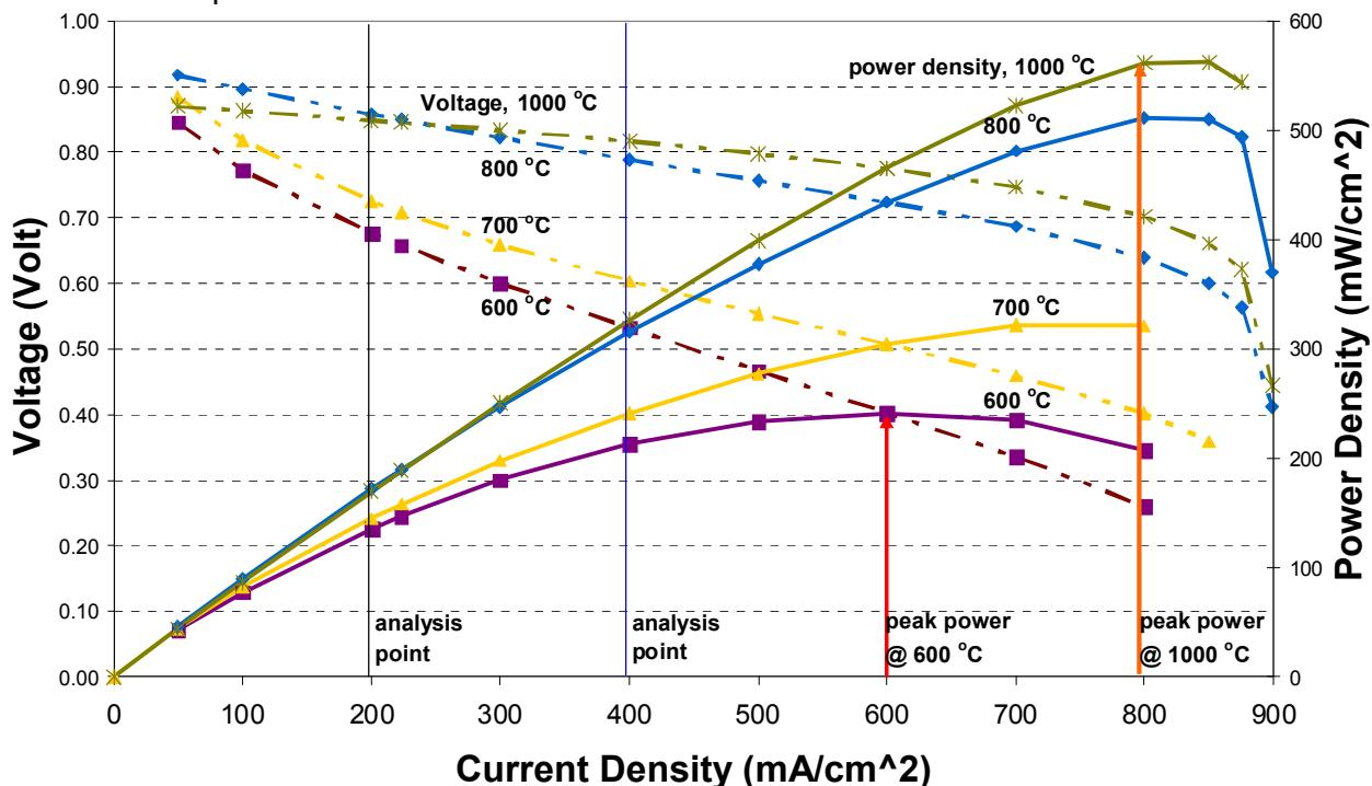
1) cell operation and 2) system-wide heat transfer. For example, for non-ideal cell operation, the excess heat is greater at higher current density due to greater voltage loss. The benefit of
