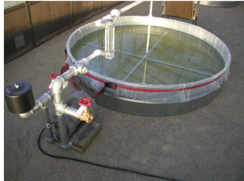
Six-foot diameter algae growth tank with Air/CO 2 blower assembly in outdoor greenhouse facility at SNL/NM.
