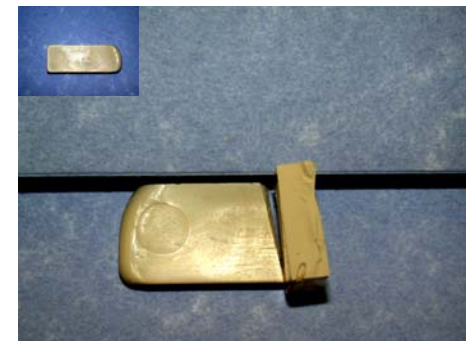
Short shot at 140°C, 100% speed, 50% pressure, 75% fill
