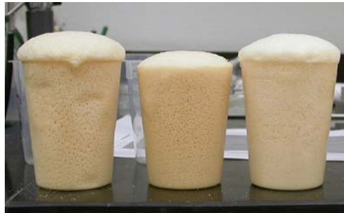
Mixing protocols change foam density and microstructure
