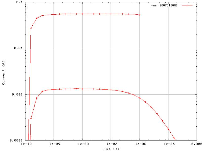
FIG. 2: The top curve shows transient current as a function of time for a bias voltage 300 V. The radiation pulse duration is  $10^{-6}$  s. The lower curve shows the depolarization current during subsequent irradiation with no bias. This current flows until the sample is depolarized.
