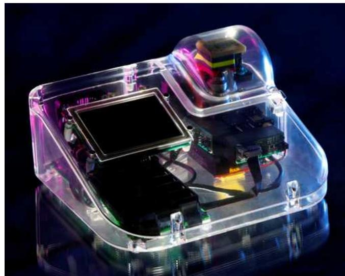
Sandia's RapiDx can analyze drops of blood or saliva in a doctor's office, enabling low-cost, rapid diagnoses during an office visit.
