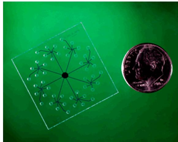
RapiDx processes and detects protein signatures by conducting each sample -processing and -analysis step within a microfluidic chip.
