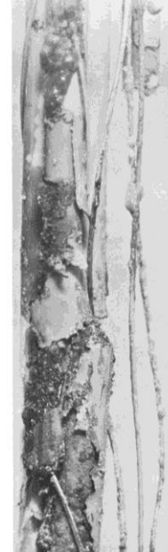
Mid-section of damaged fuel bundle
