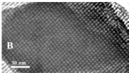
Fig. 2 TEM images of sample e with cubic mesostructure: (A) [111] direction; (B) [100] direction. Inset is electron diffraction pattern for A.
