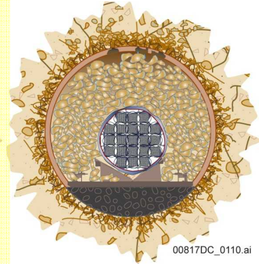
(c) After Drip Shield Plate Failure
