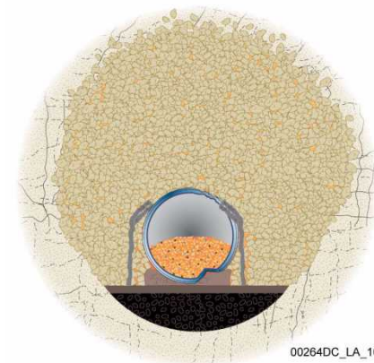
(c) After Drip Shield Plate Failure
