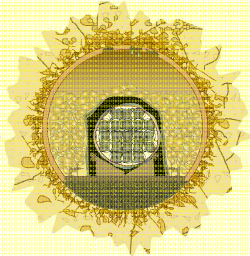
(b) After Drip Shield Framework Failure
