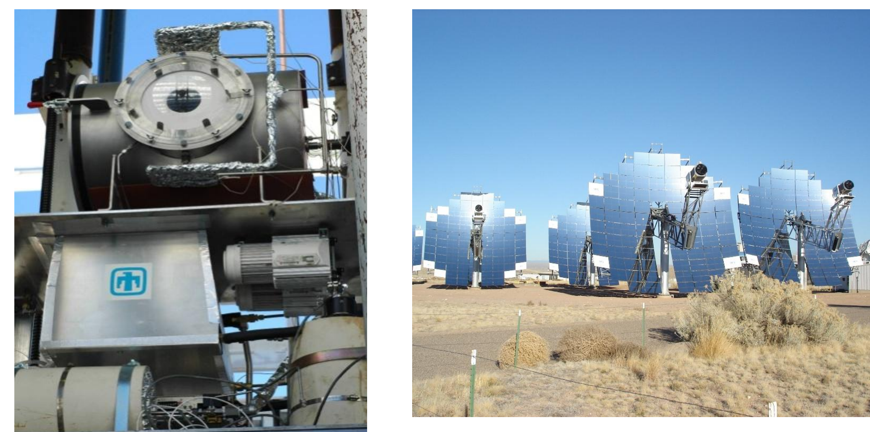
Fig 2. CR5 chemical heat engine prototype for CO 2 and H 2 O splitting (shown for CO 2 ). High utilization of reactive structures and heat recuperation contribute to an anticipated 20% solar-to-chemical conversion efficiency. Our goal is to develop and demonstrate an advanced 9 kW th heat engine.
