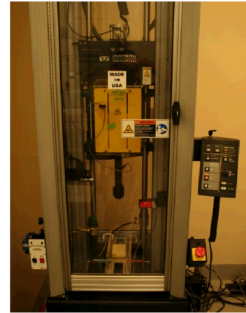
Drop-weight impact tester
