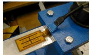
Array of piezoelectric ceramic sensors and actuators
