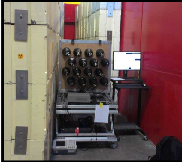
Neutron Scatter Camera, 32 elements
