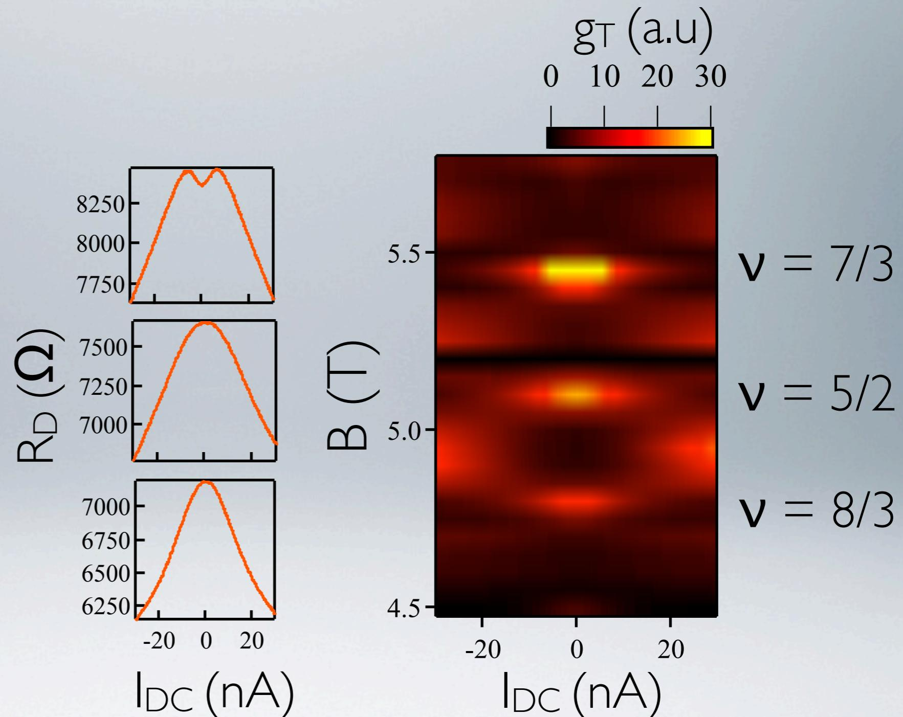
Tunneling I-V curves can provide useful information about the quasiparticles
