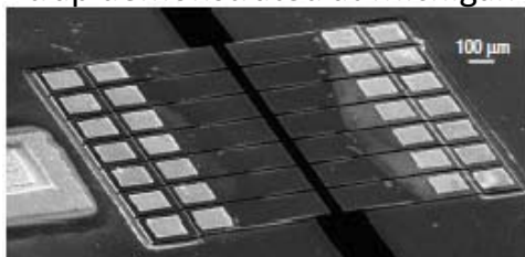
Lithographically fabricated GaAs trap demonstrated at Michigan
