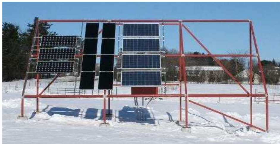
Three PV Systems under study at UVM: two crystalline silicon and one thin film. Data collection to commence in April, 2011
