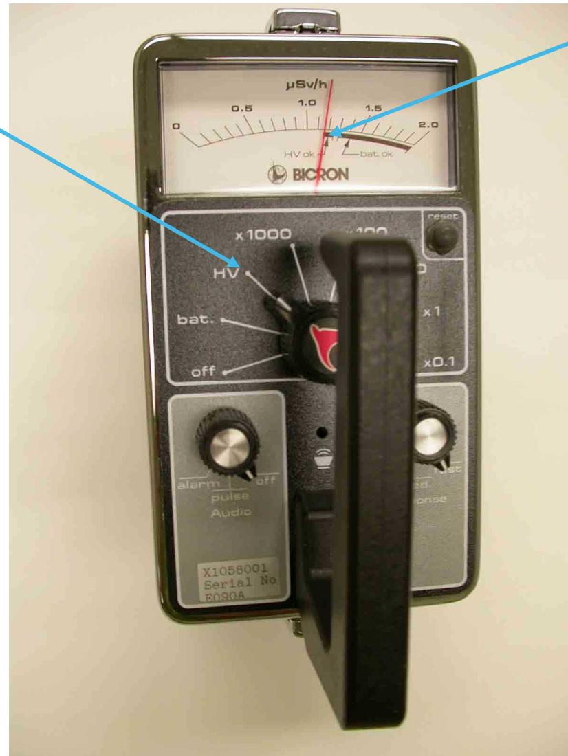
Reading should be within the “HV ok” range
